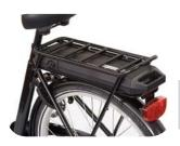
To disconnect the battery, unlock the battery lock with the battery key clockwise. Then remove the battery from the controller box by pulling the handle at the bottom of the battery.
