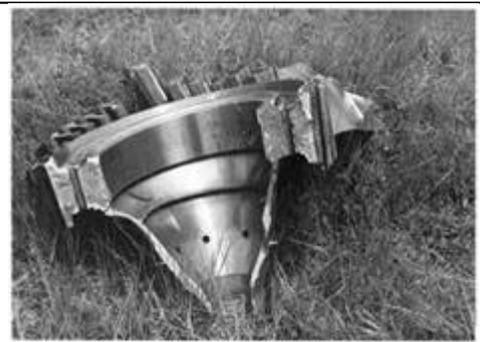
Damage caused to aircraft hull and engine from fan disc failure in the Pensacola incident
